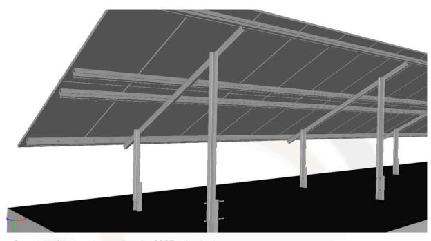
Supporting frame and grounding pile: S235 galvanized
